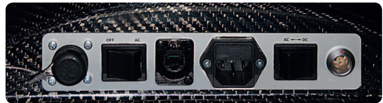
LAN-cable Mains Fuses DC
